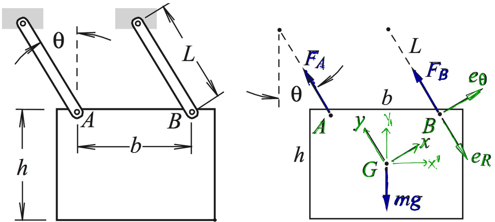
Because of the geometry of this system (4-bar with equal-length, opposite links), the body only translates.
