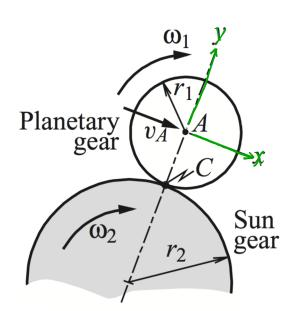
We know that A will follow a circular path of radius  $r_1+r_2$ So,  $\overline{V}_A = V_A \overline{c}$  and  $\overline{O}_A = \overline{V}_A \overline{c} - \frac{V_A^2}{r_1 r_2} \overline{c}$
