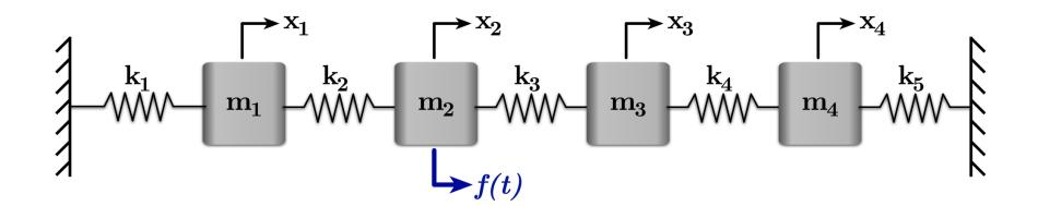
The forced mass of an n-mass system has a zero-magnitude response at n-1 frequencies.
