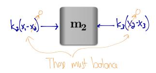
Notice that we have forces to the left and 2 DOF to the right. So, we have two frequencies at which m2 can be stationary.
