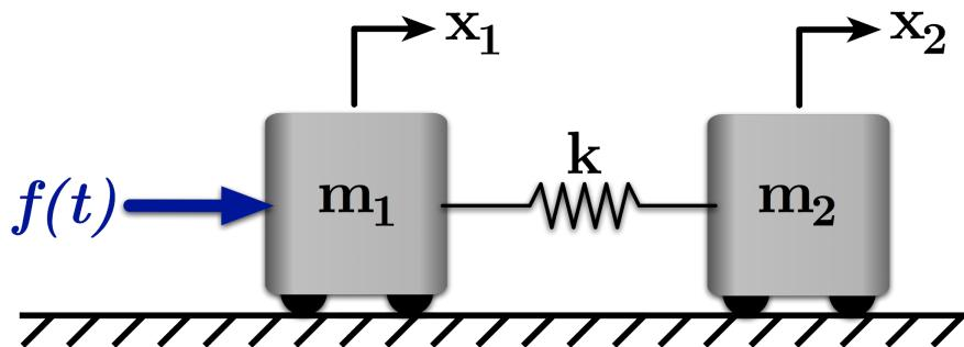
Q: What should  $f(t)$  be to move  $x_1 \rightarrow x_{1d}$  and  $x_2 \rightarrow x_{2d}$  as quickly as possible?
